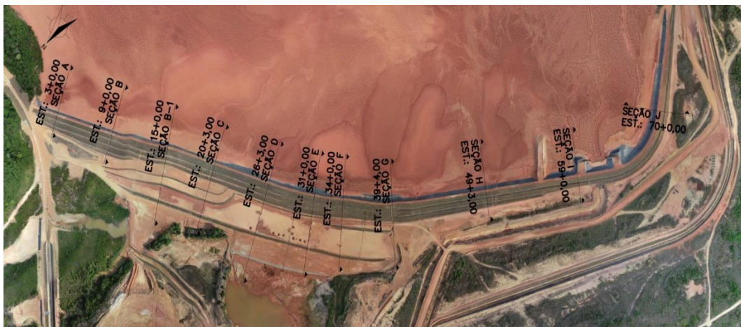
Figure 1. Sections B1 dam, Hydro Paragominas.
